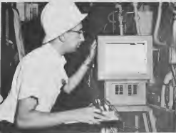
Robert E. Levy of Esso Research & Engineering while on a 3-week assignment at Lago uses this high speed temperature recorder to conduct dynamic tests at the PCAR. The data obtained will be used to provide improved control of PCAR operations from the new Refining Controlhouse.
